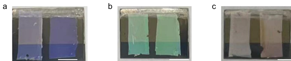
Figure S25. Photographs of flexible blue, green, and red light responsive PeLC-PDs. The devices were fabricated by simply sticking the individual LC polymer films onto the incident side of the perovskite photodiode. Scale bars: 5 mm. Related to Figure 5.
